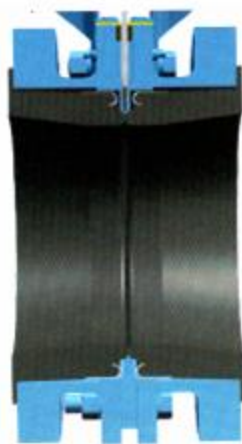
Valve in the fully open position
