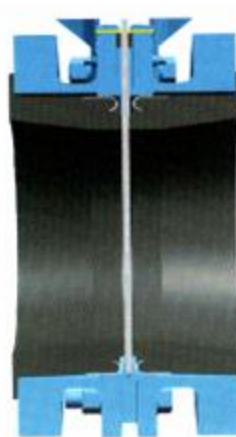
Valve in the fully closed position
